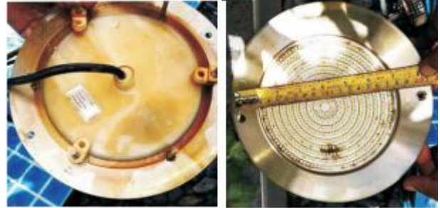
No protection circuit, easy to burn the LEDs
